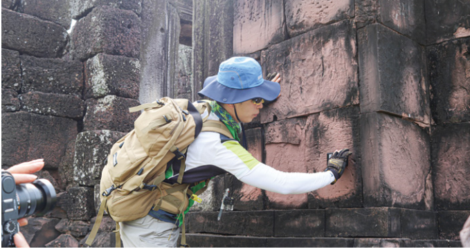
6 Investigation of Prang Hin Daeng - Measuring weathering rates of stone
